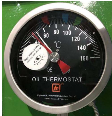
Figure 8-4 Oil surface temperature controller
