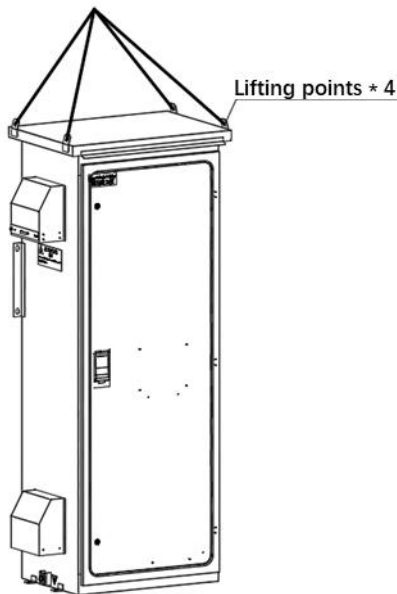
Fig. 5-4 Hoisting schematic drawing of the standardized Auxiliary panel
