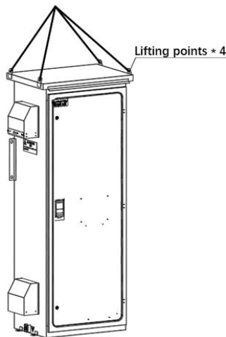
Fig. 5-4 Hoisting schematic drawing of the standardized communication power cabinet
