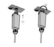
floating screw counterclockwise as shown in the figure below. After removing the stick, tighten the anti-dust cap clockwise to ensure inverter protection.
