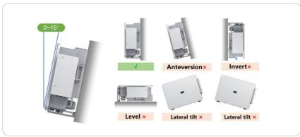
Figure 4-9 Vertical installation diagram of inverter
