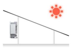
Figure 4-2 Installation Position of the Inverter
