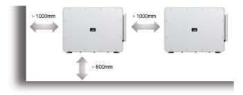
Figure 4-10 Inverter Installation Position Clearance Figure (unit: mm)
