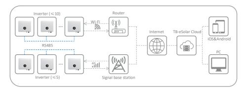
Method 1 only one inverter with the 4G/ WiFi stick, the other inverter be connected through the RS 485 cable.
