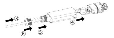
4. Insert the wiring terminal into the sealing head, adjust the communication cable, insert the sealing ring, and lock nut.
