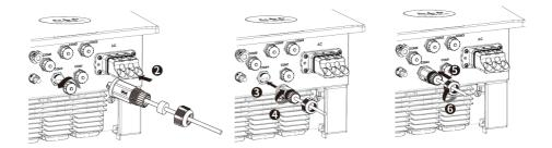
Connect the network cable to NS protection device
