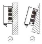
7. Never install the inverter horizontally, or with a forward tilt or with a backward tilt or even with upside down. The horizontal installation can result in damage to the inverter.
