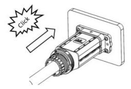
5. Tighten the nut with an open-ended wrench and complete the installation with a "click, click, click", then complete the installation.
