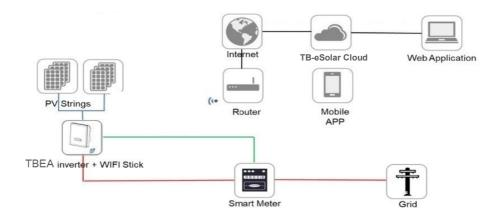
The smart meter should support the MODBUS protocol with a baud rate of 9600 and address set 1. Smart meter as above SDM630-Modbus connecting method and setting baud rate method for modbus please refer to it's user manual.
